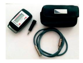
The **MEGADYNE DTM-MICRO** is used to determine the tension of a drive belt, by measuring the frequency of the static belt.
