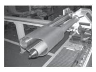
Designed for cutting individual Timing Belts as well as V-Ribbed Belts from the sleeve.
