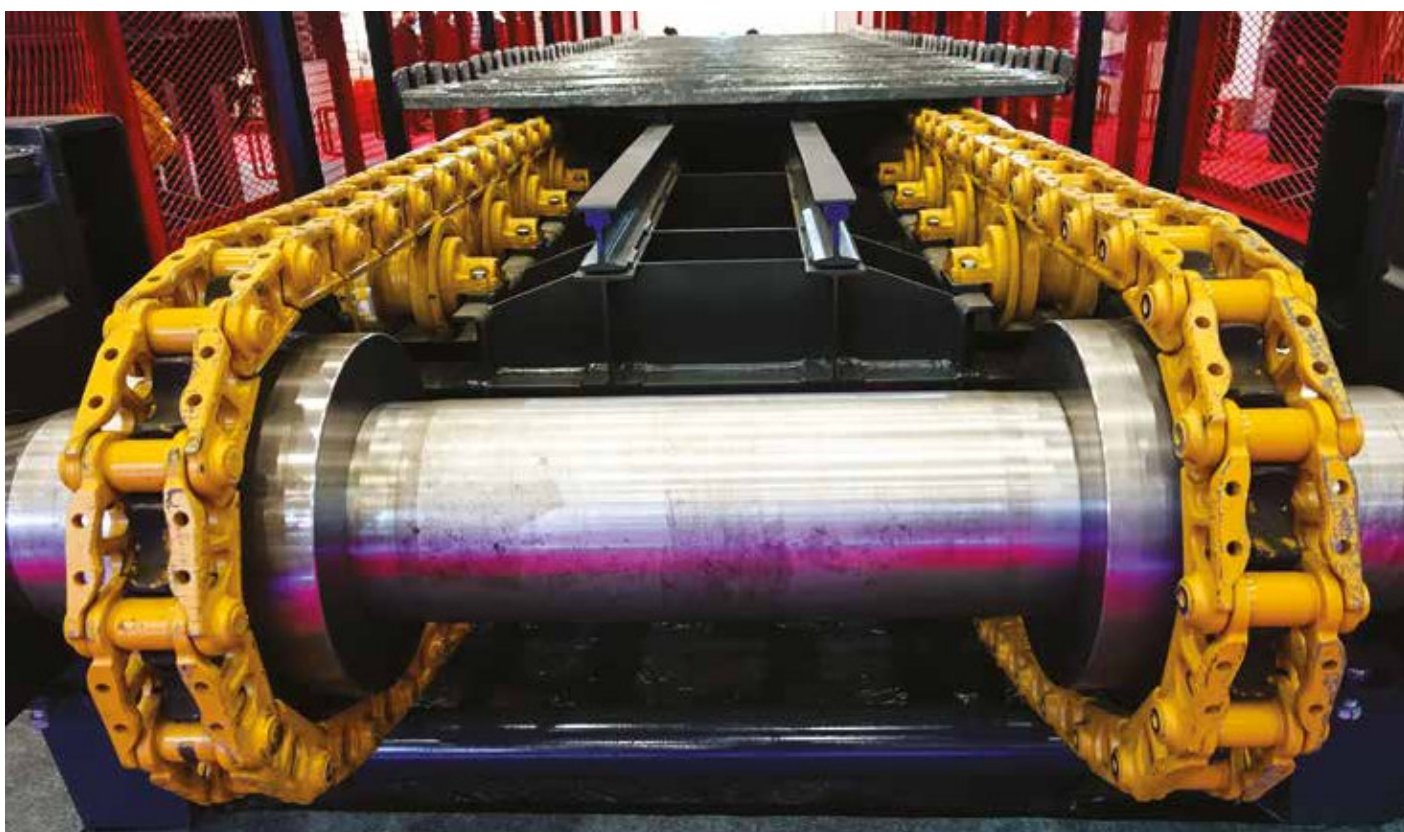
Locking conveyor chain wheels using SIT-LOCK® 4 COMPACT.
