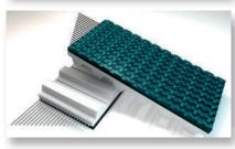
**SUPERGRIP PETROL** - PVC Cover with high CoF, applicable for slight height compensation, low shock absorption capabilities. Improved adhesion even in case of moisture and dirt - for incline, feed and take-a-way conveying applications. Seamless weldable on Megalinear and Megaflex.
